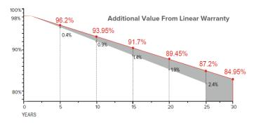
For PERC Monocrystalline Modules, the maximum loss of power output from the Peak Power at STC at
